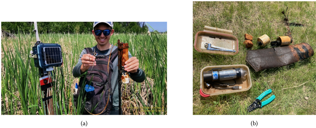
Fig. 3. (a) Spudnik that failed from beaver chewing its wires (b) Onset HOBOT datalogger after being removed from the sandy river
